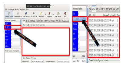
**Figure 8:** Comparison of before and after DHCP starvation attack.
